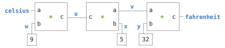
In this figure, we see on the left a multiplier box with three terminals, labeled a, b, and c. These connect the multiplier to the rest of the network as follows: The a terminal is linked to a connector celsius, which will hold the Celsius temperature. The b terminal is linked to a connector w, which is also linked to a constant box that holds 9. The c terminal, which the
